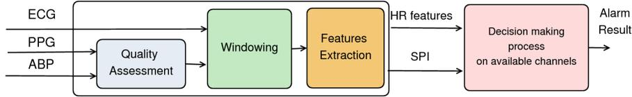
Figure 1. The general framework to determine the validity of an alarm.
